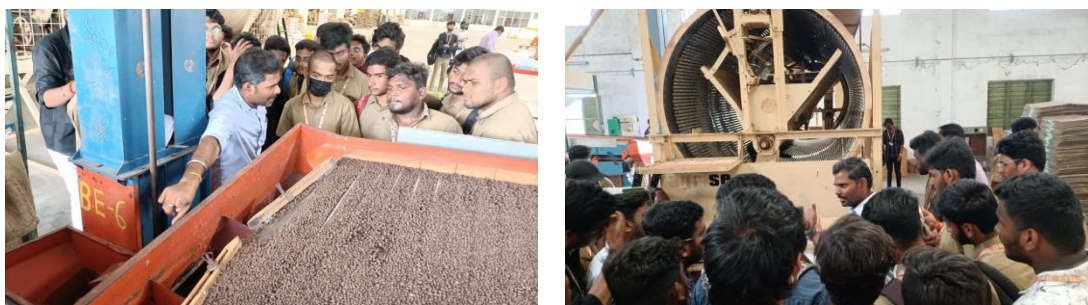
Process of Cleaning & Grading by using Gravity separator & Needle Sorter
